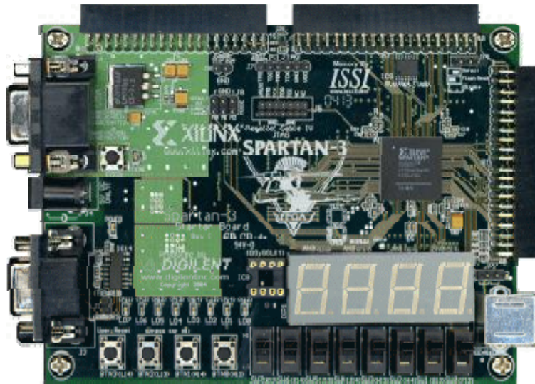
Fig: Xilinx Spartan 3 Board, used for hardware testing of cores
